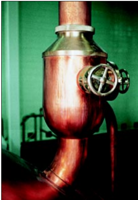
A close-up of the entry port valve on one of the new copper kettles.
