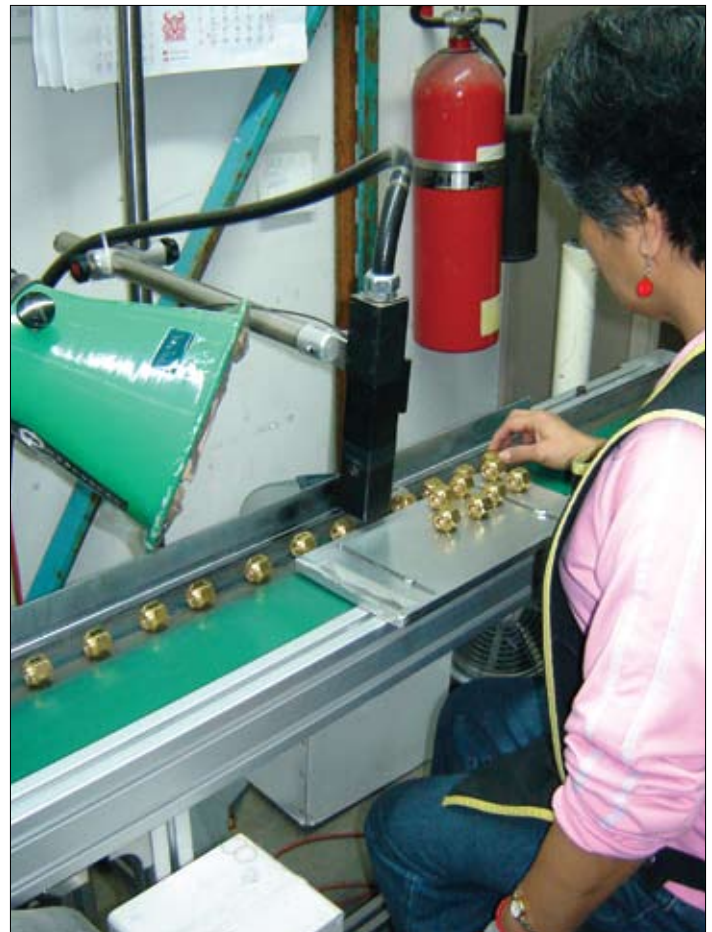
Feeding the forged flare nuts into the marking machine.
