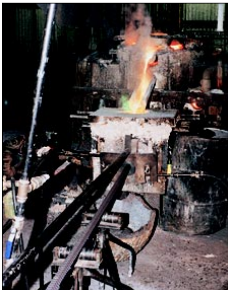
Continuous casting of hexagonal bronze bar.
